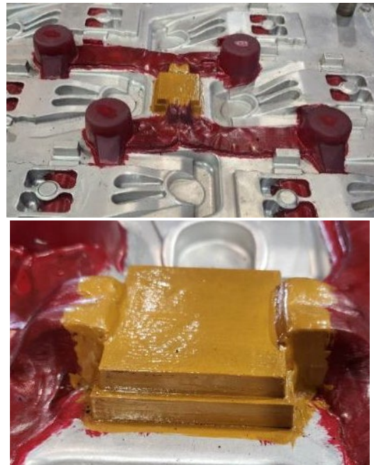
Figure 12. The 3D printed pattern pieces with the 0.5" well inserted onto the machined plate are shown.
