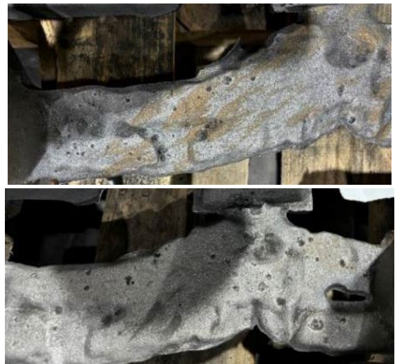
Figure 23. The cope side of the generated runners poured in the physical trials. Slag inclusion indications are present in the top of the runner.
