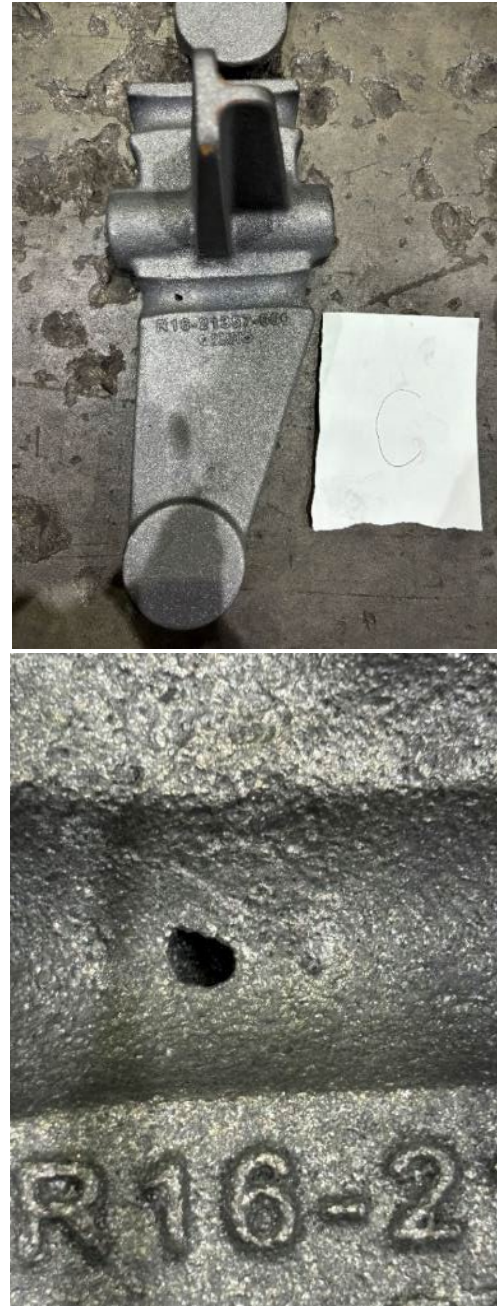
Figure 20. The casting produced with generative gating that was rejected due to a negative indication. Left: The complete casting. Right: A close-up of the defect.
